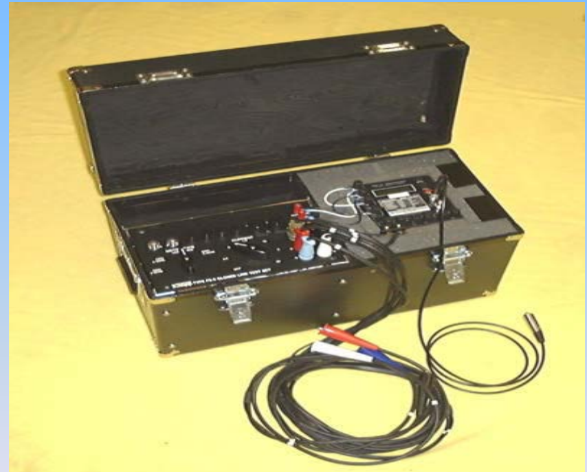
Closed-Link test system used with watt-hour standard
